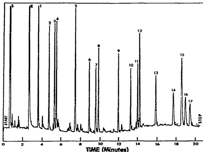
Fig. 1. Chromatogram of the permethylated cytokinins on a 12 m × 0.20 mm I.D. methyl silicone fluid fused-silica capillary column programmed from 180 to 260°C at 6°C/min. NPD, each peak contains 26 pg of the cytokinin. Peaks (for abbreviations see Table I): 1 = 2iP; 2 = DHZ; 3 = cZ; 4 = tZ; 5 = ms2iP; 6 = msDHZ; 7 = mscZ; 8 = mstZ; 9 = IPA; 10 = DHZR; 11 = cZR; 12 = tZR; 13 = msIPA; 14 = msDHZR; 15 = OHBAR; 16 = mscZR; 17 = mstZR; R = reagents; S = solvent.
